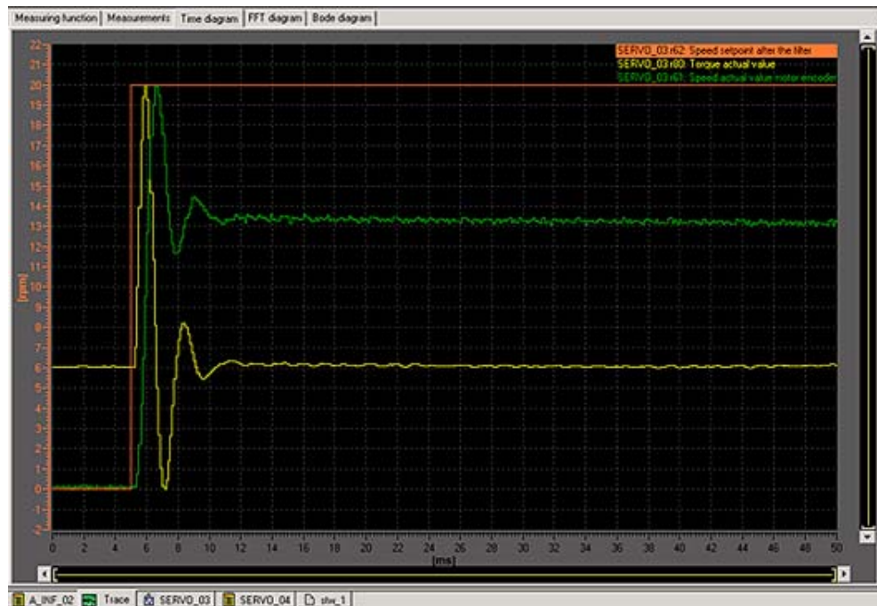
Figure 7-59 Measurement with modified P-gain
