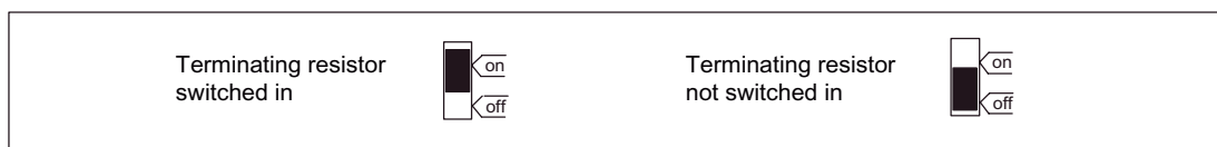
Figure 4-7 Terminating resistor switched on and off
